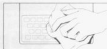
1. Make sure the original keyboard is clean and check that all the keys function.
